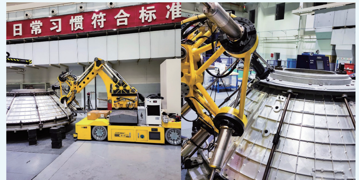
In-situ machining of Tianzhou-6’ conical segment
